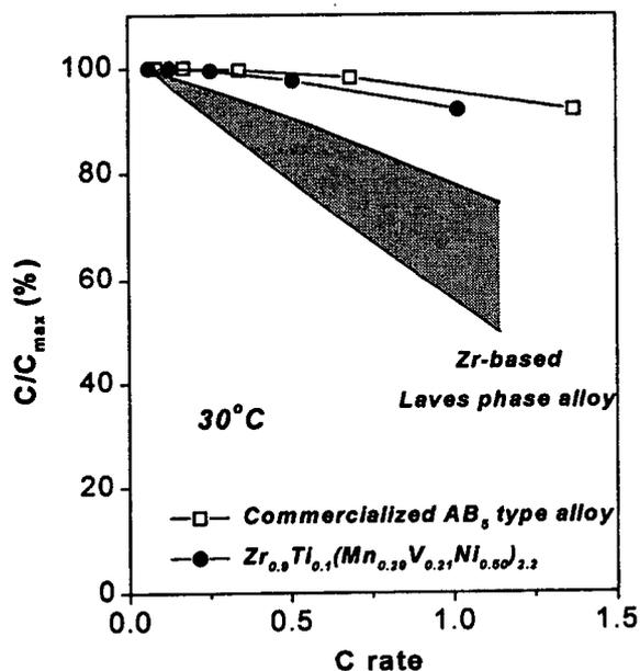
Fig. 4. Rate capability of  $Zr_{0.9}Ti_{0.1}(Mn_{0.29}V_{0.21}Ni_{0.50})_{2.2}$  and commercialized  $Mm(Ni-Co-Al-Mn)_5$  alloys at  $30^\circ C$ .
