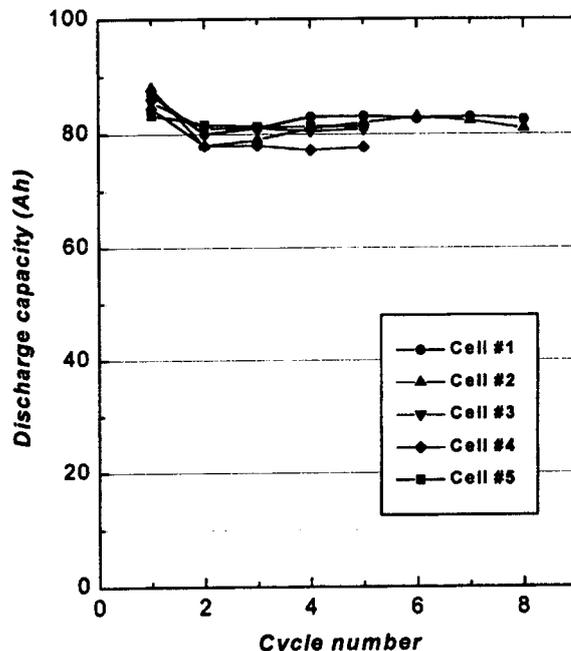
Fig. 6. The activation behaviours of proto-type 80Ah cells after hot-immersion and slow-charging treatments.
