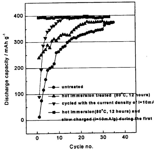
Fig. 5. The activation behaviours of Zr-based alloy electrode after various treatments.
