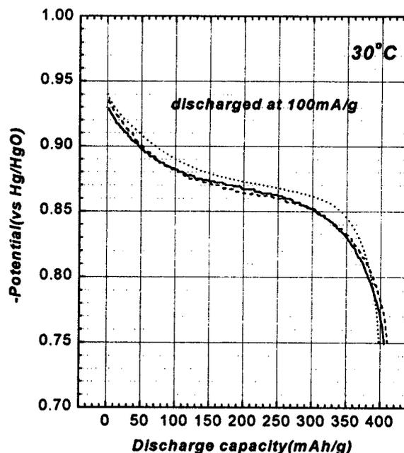
Fig. 2. The discharge curves of various hypo-stoichiometric Zr-based alloy with optimized composition.
