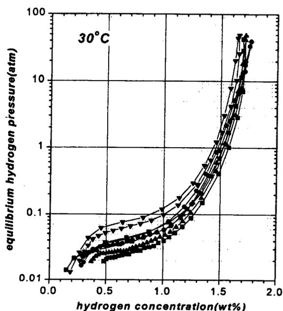
Fig. 1. The P-C-T curves of various hypo-stoichiometric Zr-based alloy with optimized composition.
