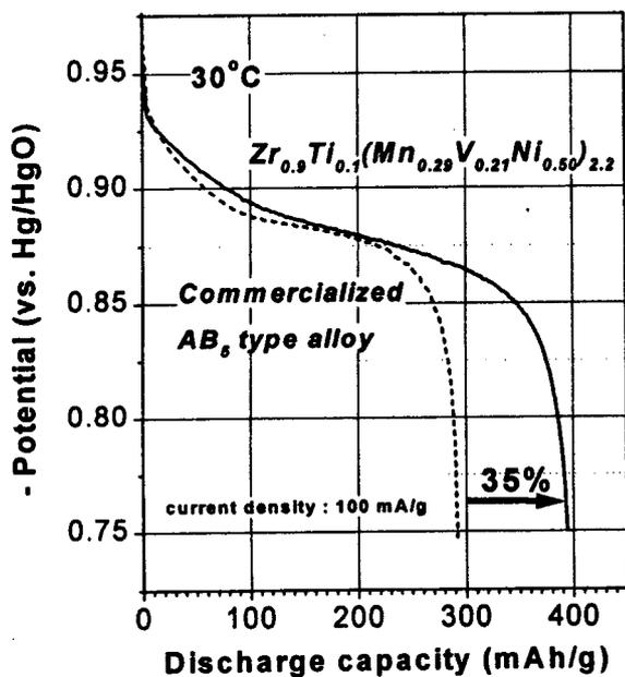
Fig. 3. Discharge curves of  $Zr_{0.9}Ti_{0.1}(Mn_{0.29}V_{0.21}Ni_{0.50})_{2.2}$  and commercialized  $Mm(Ni-Co-Al-Mn)_5$  alloys at  $30^\circ C$ .
